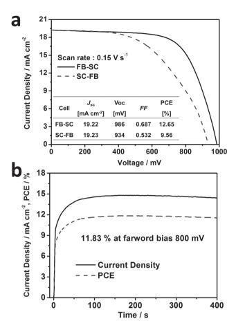
**Figure 7.** a) The J-V curves and photovoltaic parameters were performed from forward bias to short circuit (FB–SC) and from short circuit to forward bias (SC–FB) at a scan rates of 0.15 V s<sup>-1</sup> for the PSC based on  $TiO_2-TiCl_4(2)$ . b) Steady-state current measured at forward bias 800 mV and stabilized power output under simulated AM 1.5G sunlight of 100 mW cm<sup>-2</sup>.
