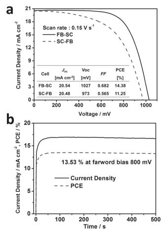
**Figure 4.** a) The J-V curves and photovoltaic parameters were performed from forward bias to short circuit (FB–SC) and from short circuit to forward bias (SC–FB) at a scan rate of 0.15 V s<sup>-1</sup> for the PSC based on  $SnO_2-TiCl_4(2)$ . b) Steady-state current measured at forward bias 800 mV and stabilized power output under simulated AM 1.5G sunlight of 100 mW cm<sup>-2</sup>.
