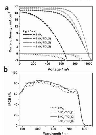
**Figure 2.** a) The J-V curves of typical planar perovskite solar cells based on a  $SnO_2$ -based ETM layer with or without  $TiCl_4$  treatment measured under illumination (solid) or in dark (hollow). b) Incident photon-to-current conversion efficiency (IPCE) of typical perovskite solar cells.
