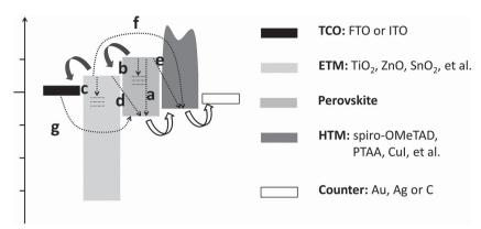
**Scheme 1.** A schematic diagram of device structure for mesoporous and planar PSCs (except perovskite/PCBM structure). The compact and/or mesoporous electron transport materials are considered as the electron transport layer (ETL). The electron and hole transfer processes are indicated by arrows.
