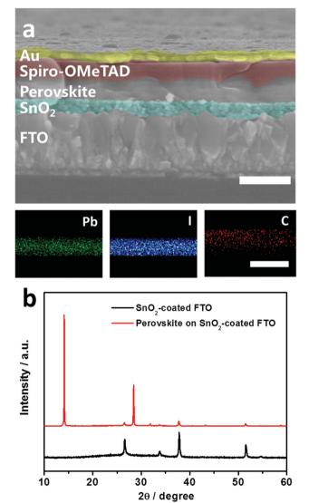
**Figure 1.** a) The color-enhanced cross-sectional SEM micrograph and energy dispersive spectroscopy (EDS) mapping of typical PSC based on  $SnO_2$ -coated FTO. Here the scale bar corresponds to 500 nm. b) XRD patterns of  $SnO_2$ -coated FTO (black) and coating with perovskite (red).
