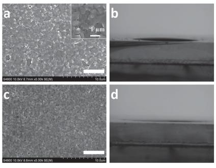
**Figure 3.** Top-view SEM images of perovskite films coated on a) FTO–SnO<sub>2</sub> and c) FTO–SnO<sub>2</sub>– TiCl<sub>4</sub>(2). Here the scale bar corresponds to 5  $\mu$ m. b) DMF contact angles of SnO<sub>2</sub> and d) SnO<sub>2</sub>– TiCl<sub>4</sub>(2) samples by putting a drop of DMF on the substrates with syringe needle of 0.26 mm.
