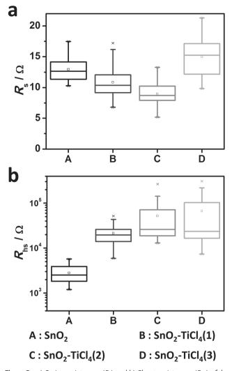
**Figure 5.** a) Series resistances ( $R_s$ ) and b) Shunt resistances ( $R_{hs}$ ) of the PSCs based on various SnO<sub>2</sub> electron collection layer.
